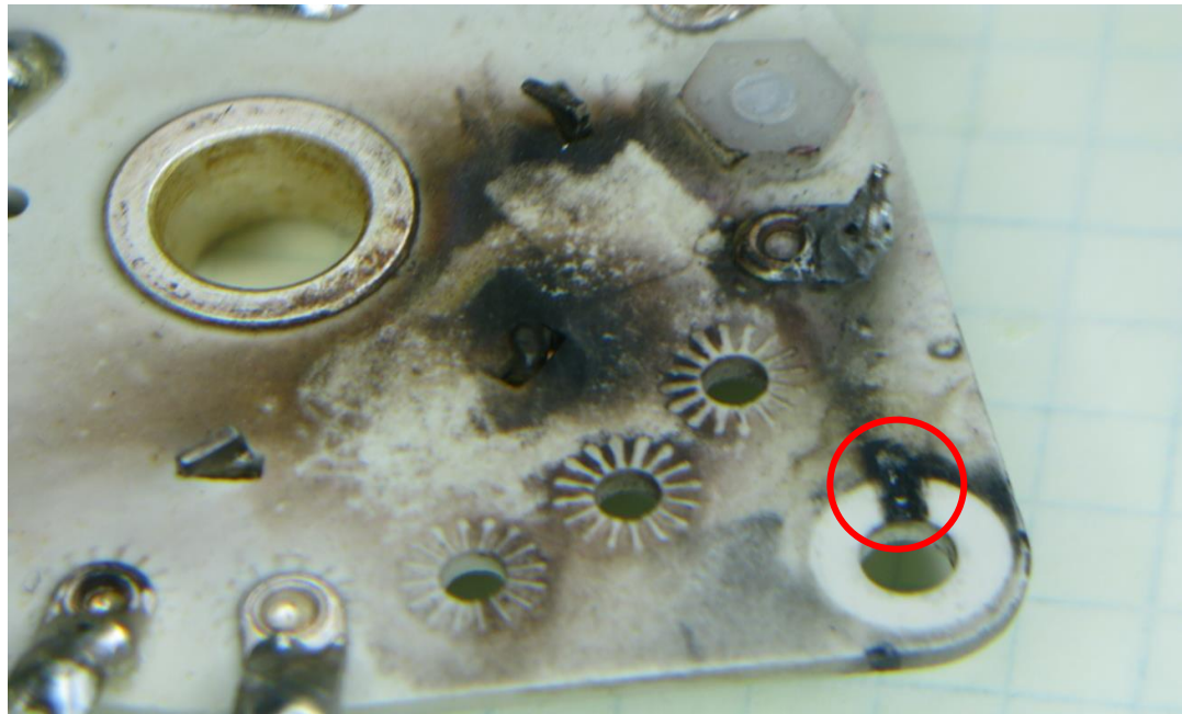
Figure 3: Arced Bandswitch in My Amplifier
