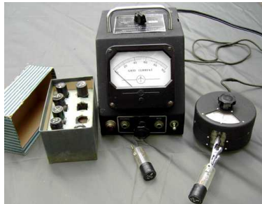
Grid Dip Oscillator (GDO)
