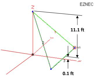
The gain of this antenna "...is only 0.25 dB less than if the antenna were in Free Space."
