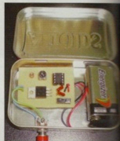
Figure 2 — Here is the completed theremin and battery all in an Altoids case.
